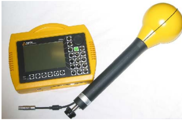
Figure B-2: Narda Selective Radiation Meter SRM-3000 with probe
