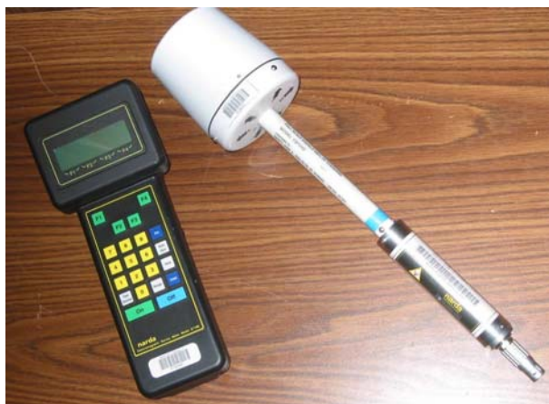
Figure B-1: Narda Electromagnetic Survey Meter 8718B with probe C8722D
