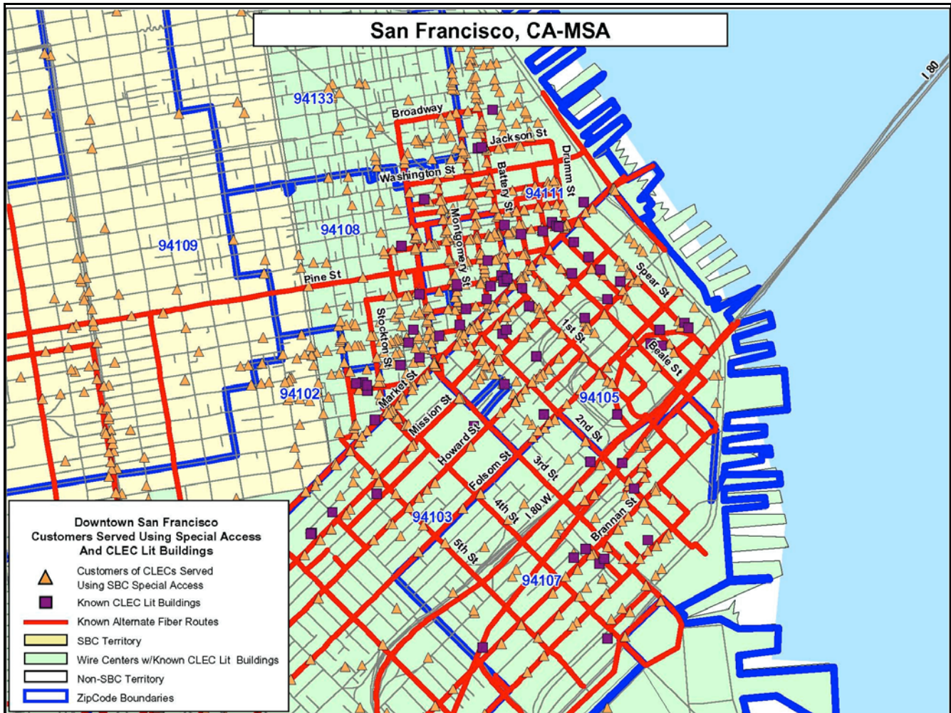
Figure 1. SBC map of Downtown San Francisco showing CLEC enterprise customers being served using Special Access and CLEC “lit” buildings.
