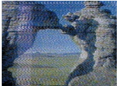
Reception of two simultaneous signals
