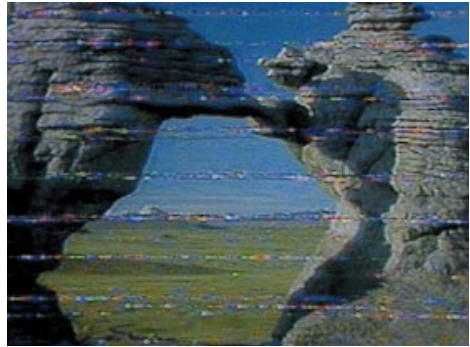
Interference caused by a motor
