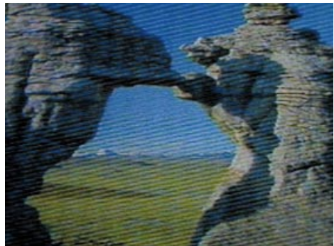
Interference caused by a radio transmitter (cable, channel 17 to 22)
