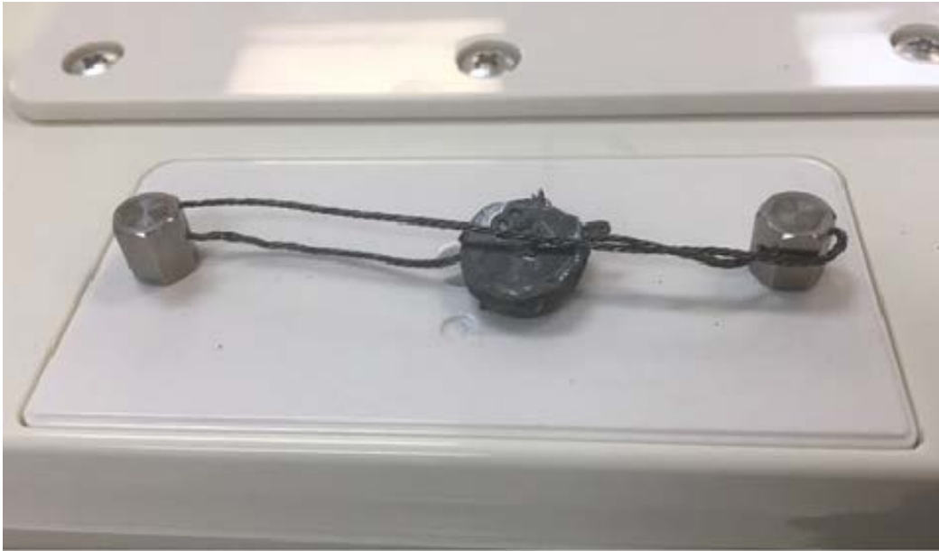
Typical Sealing / Scellage typique
