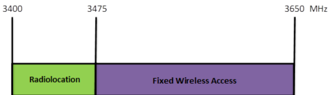
Figure 1: Current spectrum utilization, 3400–3650 MHz
