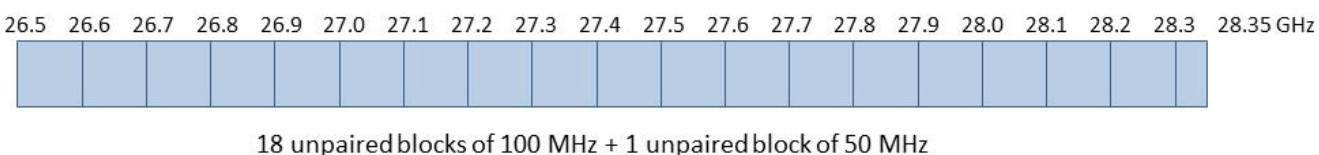
Figure 2: Canadian band plan in the 26.5-28.35 GHz frequency band
