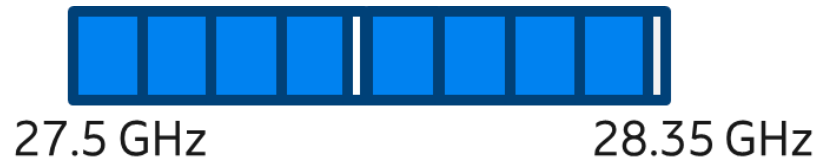
FIGURE 2: 28 GHz block structure with 100 MHz channels distributed as 2x425 MHz blocks without spectrum swapping. 9
